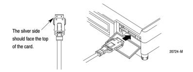
3. Attach the cable to the processor.
