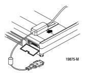
2. Attach the cable to the PCMK card.
